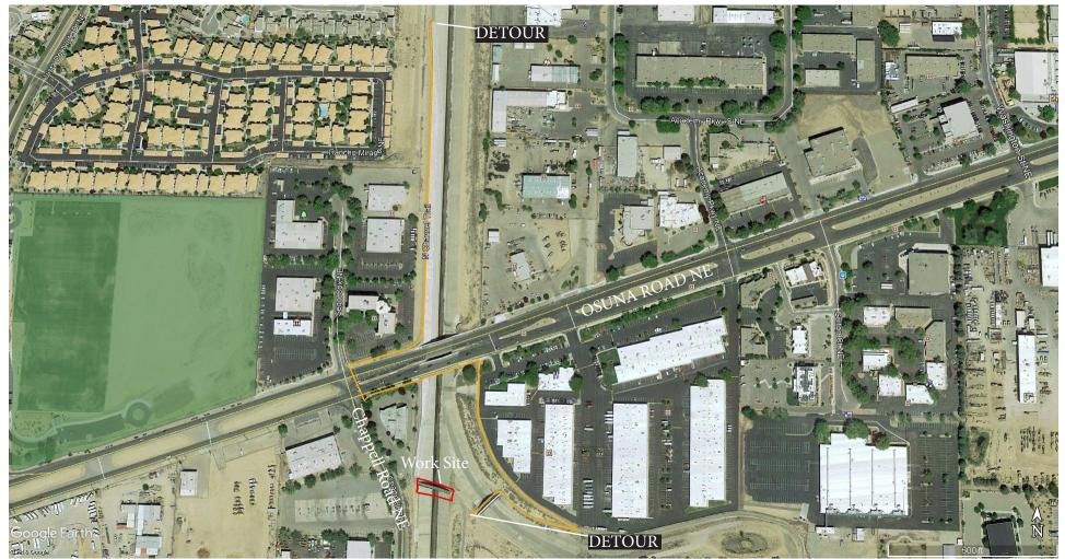
North Diversion Channel Trail Detour Work will be done on the bridge south of Osuna Rd NE over the North Diversion Channel. The wooden bridge deck will be replaced by a concrete deck.
